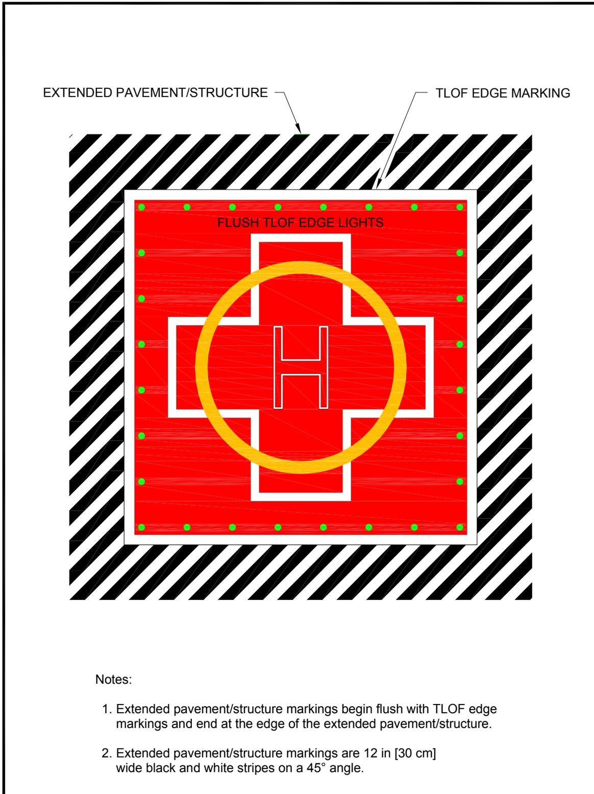
**Figure 4–26. Extended Pavement or Structure Marking: Hospital**
